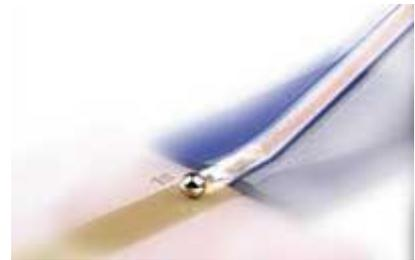
The distance covered by the steel ball starting from the lower edge of the testing device defines the
